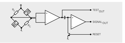
The non-tared signal is available at the output Test<sub>out</sub>. To prevent saturation of subsequent stages, Test<sub>out</sub> should ideally read between -2 V and +2 V when the sensor is installed and no load is applied. During operation this value may then be between -5 V and +5 V. The Test<sub>out</sub> output can furthermore be used to check the measuring chain. In case of an open bridge circut, Test<sub>out</sub> goes into saturation.
