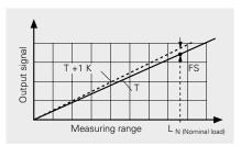
The largest temperature coefficient (TC) of output range is the largest variation in output range which occurs during a change in temperature by 1 Kelvin. It is expressed in percent of FS<sup>\*</sup>) per Kelvin.
