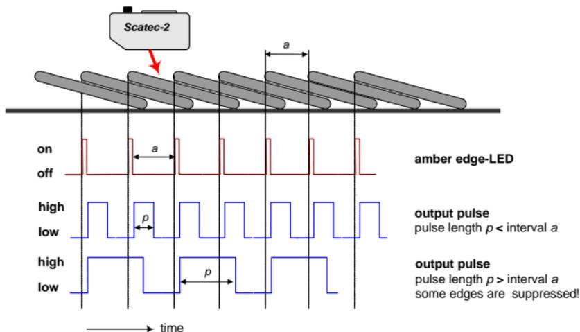
A helpful rule of thumb is: Output pulse length  $p$  in milliseconds must be shorter than 1.2 million divided by the production rate given in copies per hour
