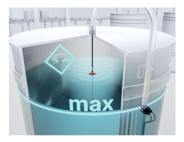
In addition to traditional object detection, fiber optics can also be used for liquid level detection. A distinction is made between contact and contactless level detection. Fiber optics for contact level detection are equipped
