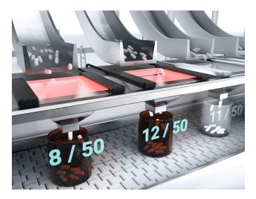
Array fiber optics are used for position-independent detection of irregular objects. Unlike fiber optics with a single, point-shaped light beam, array fiber optics generate a broad, linear light band. Depending on the width of the array fiber optics and the operating principle, the maximum detection area can be adjusted in both the x and y directions. Glass fiber optics are characterized by low signal attenuation, which allows
