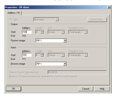
Enter the respective initial addresses. It is admissible to use Identical or overlapping addresses for output and input.
