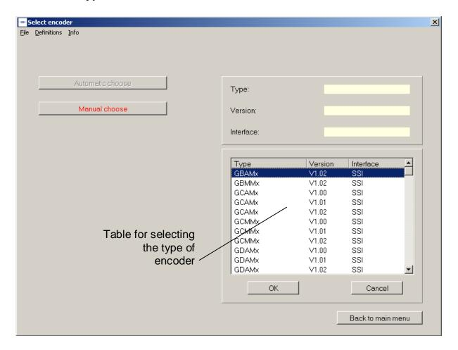
If no encoder is connected to the PC, the type of encoder can be selected from a table (manual selection). The table contains the common types. It is not only the type that is important but also the version. If your type should not be included, please contact Baumer Germany GmbH & Co. KG. Type and version can be found on the type label of the encoder.
