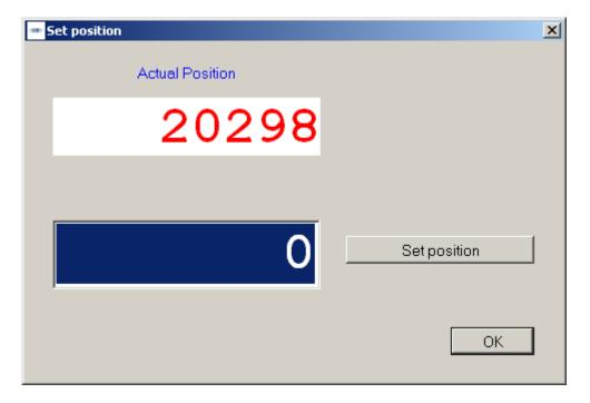
To the encoder models GXP1H, GXP1W, GXP2W with version 2C applies the following: After having assigned the preset value by the "set position" function, the external reset input must not be used.
