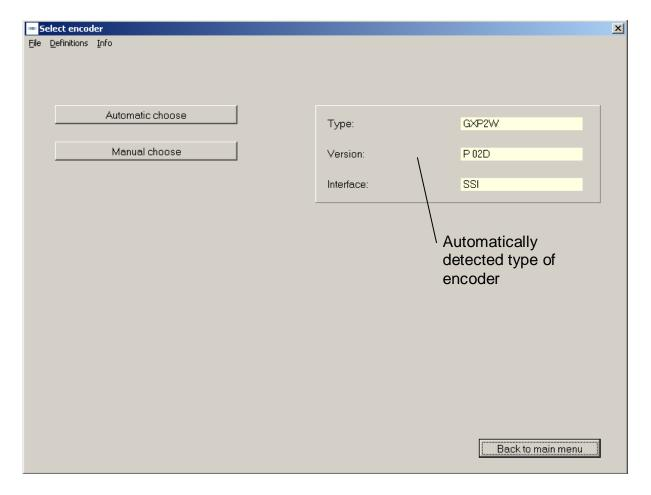
The type of encoder can be read out when the encoder is connected (automatic). This data is necessary to provide the relevant parameters for programming. If no encoder is connected or if the cable connection is not connected properly, an error message will be displayed. If the automatically detected encoder does not correspond with the encoder's type label, please contact Baumer Germany GmbH & Co. KG.
