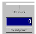
Bring the encoder to the desired start position by turning the encoder shaft. Enter the desired start value in the entry field start position, e.g. 0. Confirm entry by clicking "assign start position".
