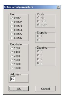
Click "settings" menu to select the serial interface COM 1 up to COM 6 to which the encoder is connected. Furthermore, you can adjust the baud rate and the address of the encoder. The other parameters such as parity, stop bits and data bits can be controlled here.
