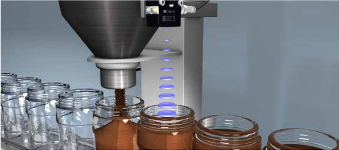
The sonic beam angle width of the new Baumer ultrasonic sensors can be adjusted on site depending on the container opening and the filling medium. A narrow sonic beam angle is necessary to measure level through a narrow opening.
