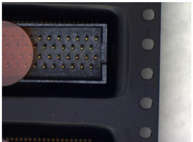
*Baumer's Design Team applied two distinctly different camera configurations to inspect the fine features of electrical connectors while also confirming they were oriented correctly in their trays as they traveled down a fast-moving production line.*
