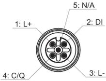
Connection: IO-Link Dual-Channel
