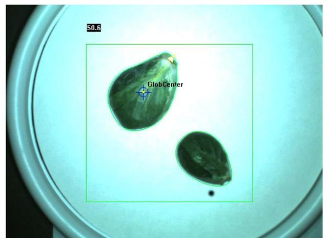
*Leveraging a GIG-E high-resolution color camera, and distributed lighting, Baumer developed a vision system to guide a high-speed delta robot arm to identify and pick the highest quality Brussels sprouts from a conveyor.*
