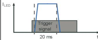
Triggered flash light with overdrive current and time-out for LED protection.
