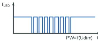
DIM (Pin2) is used as brightness control and operation mode switch. It's a high resistance current sink with 0.2 mA for 5 V and 1 mA for 24 V.
