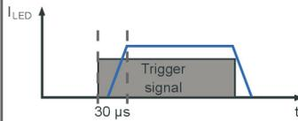
Trigger (Pin3) it is a high resistance current sink with 0.2 mA for 5 V and 5 mA for 24 V.
