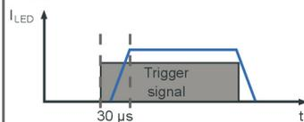
Trigger (Pin3) is a high resistance current sink with 0.2 mA for 5 V and 5 mA for 24 V.
