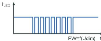
DIM (Pin2) is used as brightness control and operation mode switch. It's a high resistance current sink with 0.2 mA for 5 V and 1 mA for 24 V.
