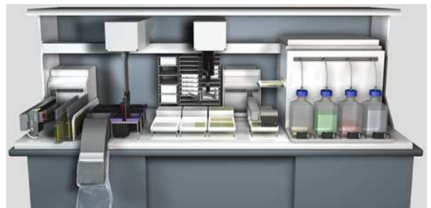
Figure 2: Liquid handling station for laboratory automation
