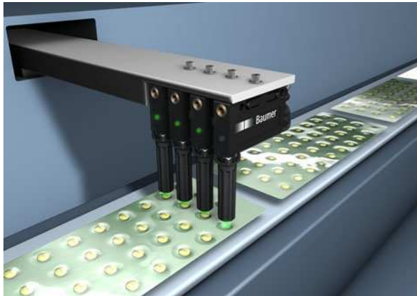
Figure 5: Ultrasonic sensors monitor the presence of tablets in blister packagings
