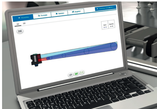
Figure 4: 3D CAD data integrating the beam path. Eased work from design-in to installation: sensor installation follows design-in and does not require any precision alignment.
